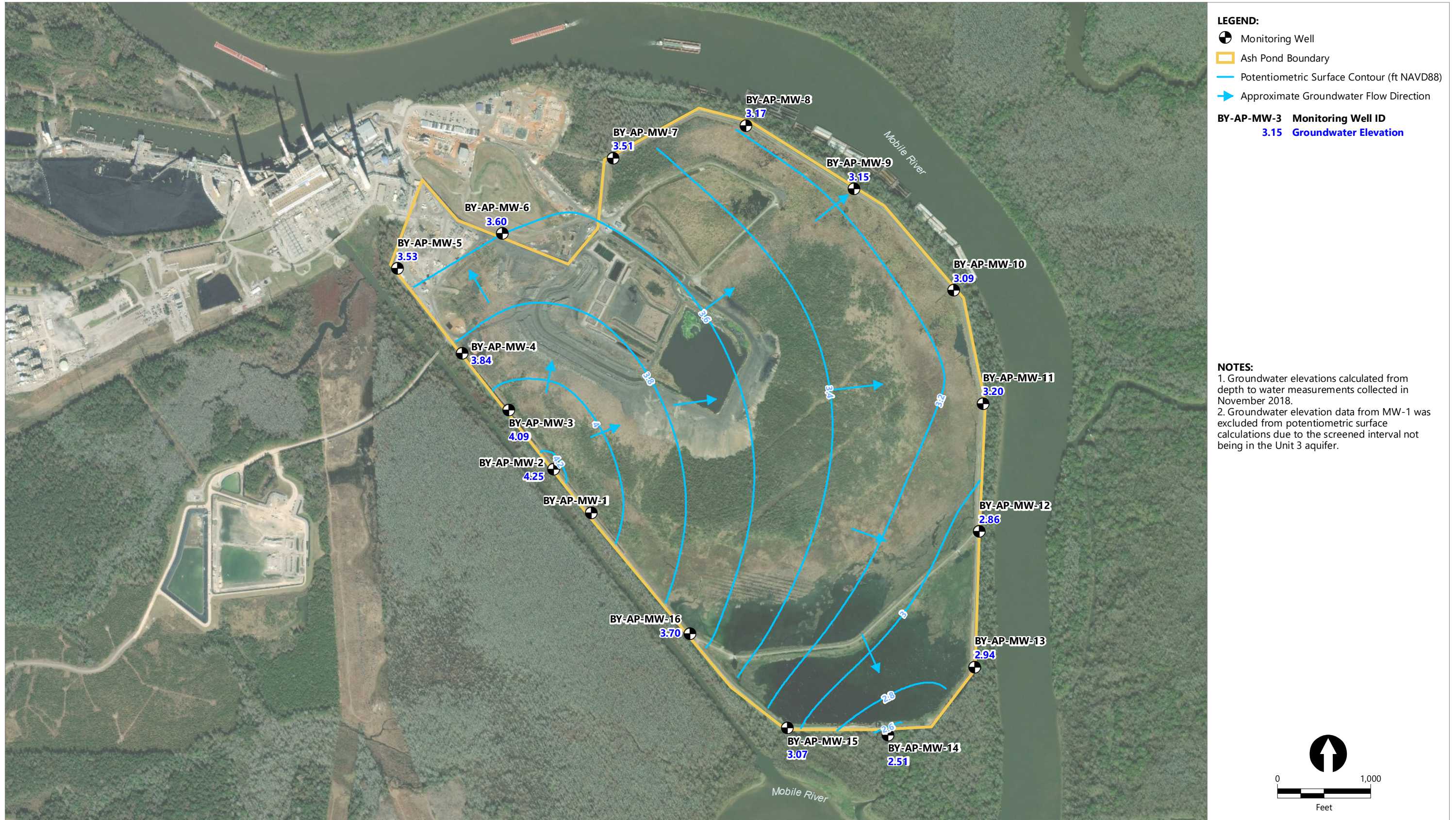
Figure 3 Potentiometric Surface Map Assessment of Corrective Measures Alabama Power Company - Plant Barry
