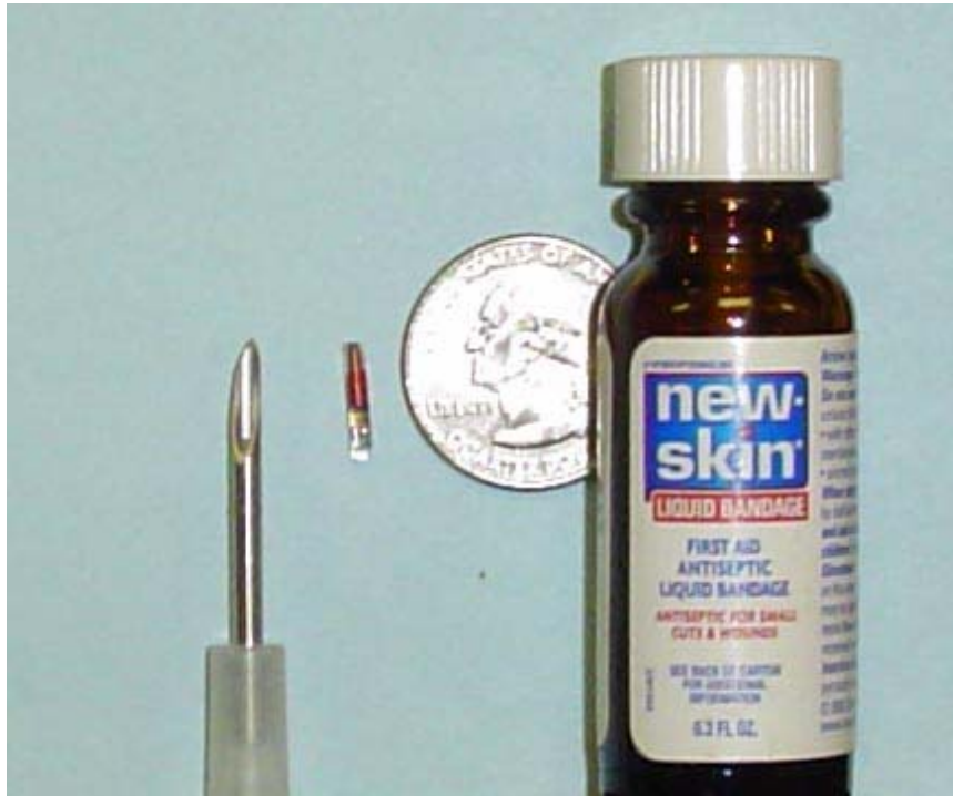
Figure 5--PIT tag injector, PIT tag, and Liquid Bandage
