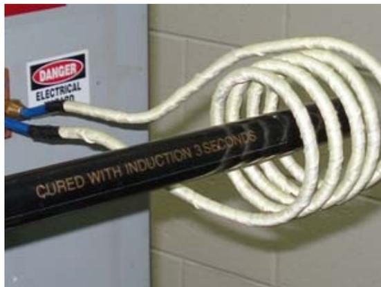
Thin wall tubing travels through a series of three induction coils.
